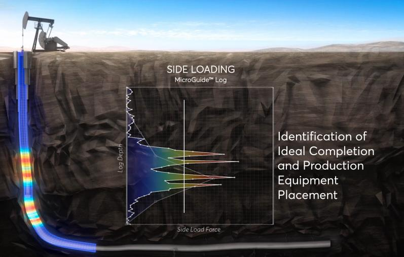
Multiple hidden areas of high side load force are identified through the use of high resolution logging.
