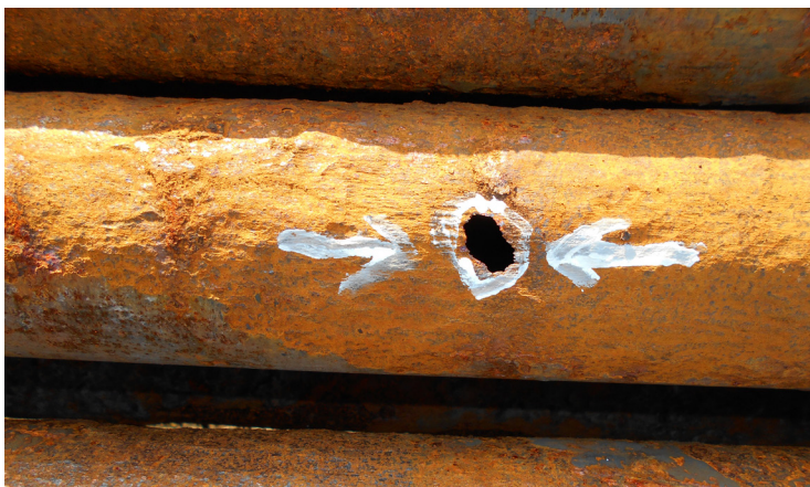
Figure 3. Tubular hole that correlates to depth identified in Figures 1 and 2.
